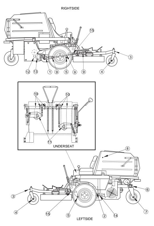
Figure 7.1 Lubrication Fitting Points
